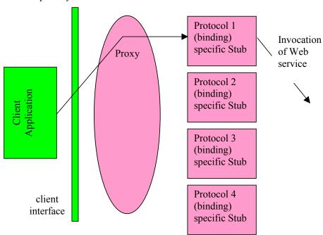
Figure 1: Possible client-side runtime architecture
